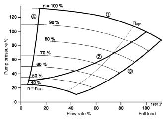
$\eta_{opt}$  Optimum pump efficiency curve
