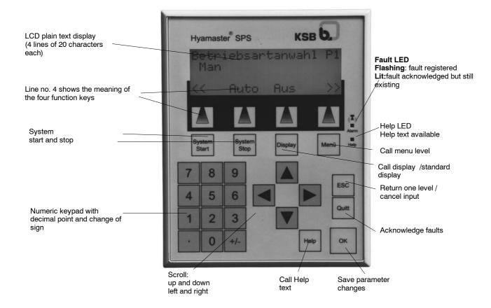
The LCD plain text display of the Operator Panel (OP7) shows operating status, parameters, help texts and faults in various levels. The first and the last function key, respectively, serve to page up and down within a level.
