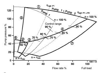
$\eta_{opt}$  Optimum pump efficiency curve
