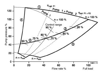
$\eta_{opt}$  Optimum pump efficiency curve
