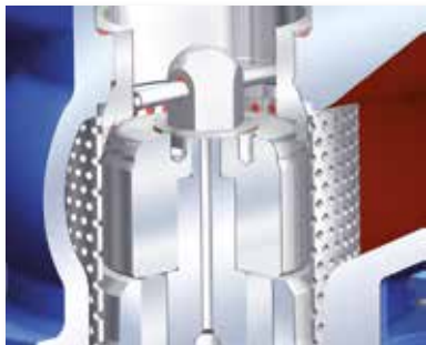
Flow divider for noise reduction
