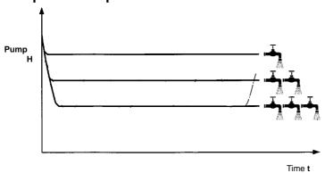
Unlike domestic water supply systems with accumulators, pumps operated with the Controlmatic E.2 control unit maintain a constant pressure at any flow rate.
